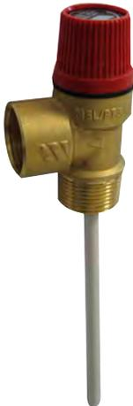
Combined temperature and pressure valve to protection tank build up. Models with threaded male/female connections or male/fitting connection for copper pipes. Nominal temperature: 92°C. Nominal pressure: 10 bar. Body CW617N, stainless steel spring, diaphragm EPDM; suitable for plumbing water.
